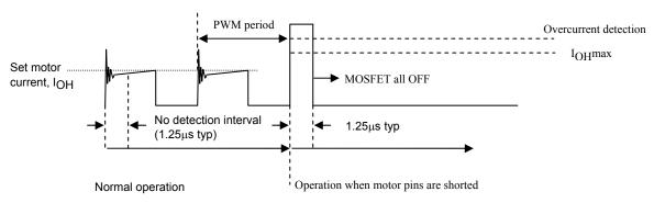
Overcurrent detection begins after an interval of no detection (a dead time of 1.25µs typ) during the initial ringing part during PWM operations. The no detection interval is a period of time where overcurrent is not detected even if the current exceeds I<sub>OH</sub>.
