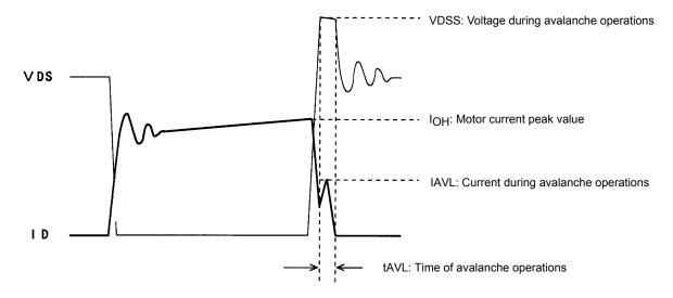
Figure 1 Output Current, ID, and Voltage, VDS, Waveforms 1 of the STK672-4\*\* Series when Driving a 2-Phase Stepper Motor with Constant Current Chopping
