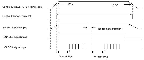
ENABLE, CLOCK, and RESETB Signals Input Timing
