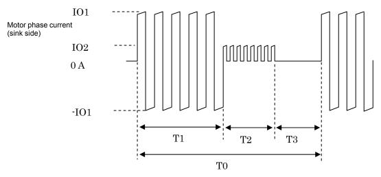
Figure 1 Motor Current Timing
