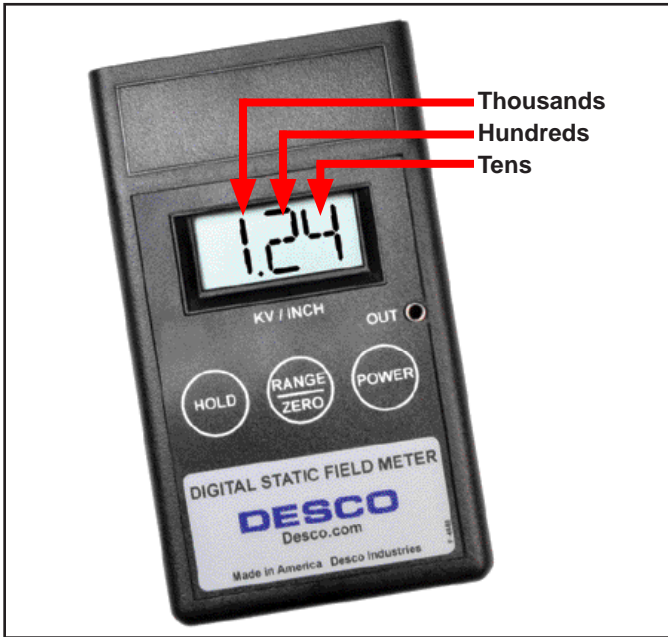
Figure 3. Reading the Digital Static Field Meter while in the \pm 20 kV range
