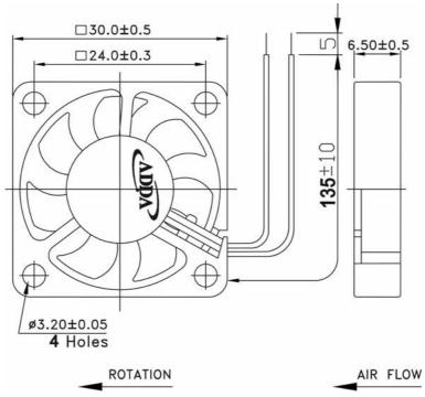
LEAD WIRES: UL 1571, AWG28, L = 135 +/- 10 mm Red = positive; Black = negative.
