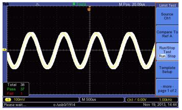
The Limit Test feature provides a guick Pass/Fail comparison between any triggered input signal and a user- defined template.
