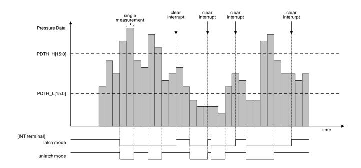
INT terminal is L at state of interrupt, and H by built-in pull-up resister at state of non-interrupt. When INT terminal is not used, built-in pull-up resister should be ON (INT\_PU\_EN=0) and the terminal should be open.
