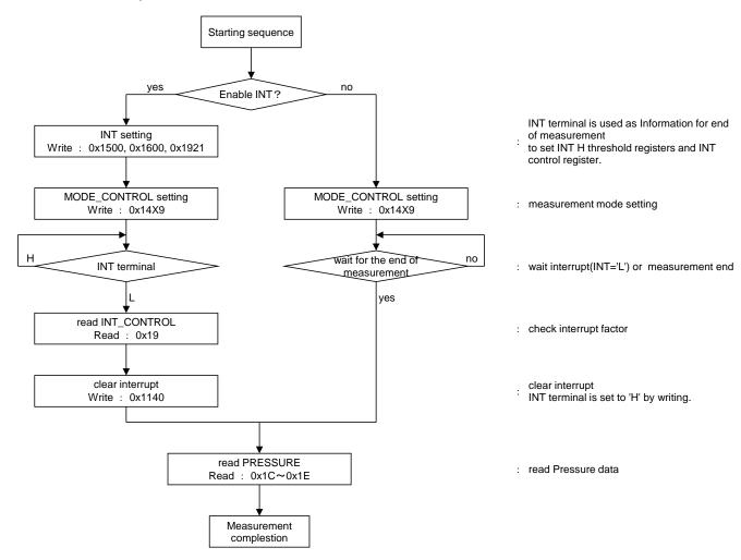
6. Measurement sequence: Continuous Mode (50ms/100ms/200ms)
