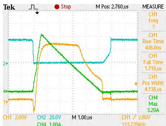
Fig 4a: Critical conduction mode
