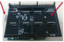
Figure 1. Connection between the Arduino and the SensorShield
