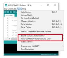
Figure 3. Board and COM Port setting
