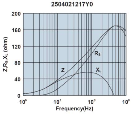
Impedance, reactance, and resistance vs. frequency.
