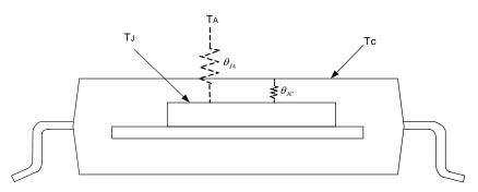
Notes: 2.  $\theta_{JA}$  should be confirmed with heat sink thermal resistance. If there is no heat sink contact,  $\theta_{JA}$  will almost be the same as  $\theta_{JC}$ .
