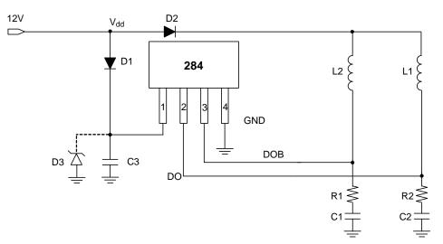
Notes: 1. Typically it is recommended to us a 56 Ohm resistor for R1 and R2 and a 2.2µF E-Cap capacitor for C1, C2 and C3. These values may need to be optimized depending on the coils used.
