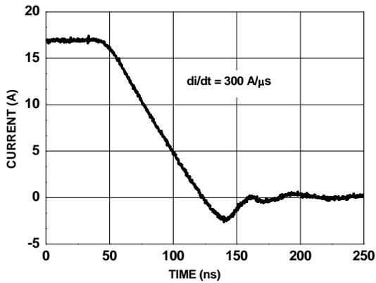
Figure 25. FDML7610S SyncFET™ body diode reverse recovery characteristic
