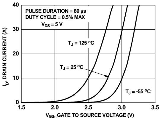
Figure 17. Transfer Characteristics
