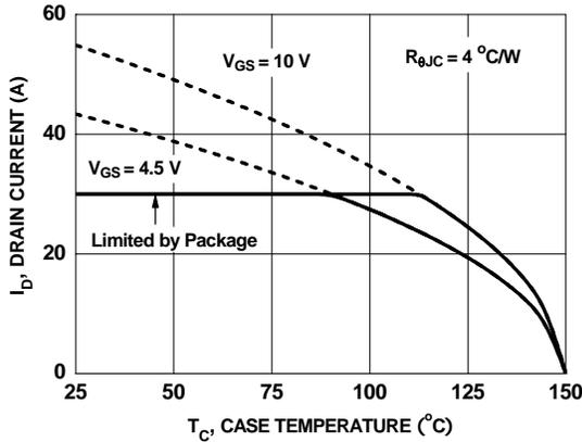
**Figure 9. Maximum Continuous Drain Current vs Case Temperature**
