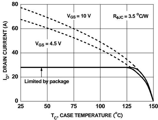
**Figure 21. Maximum Continuous Drain Current vs Case Temperature**
