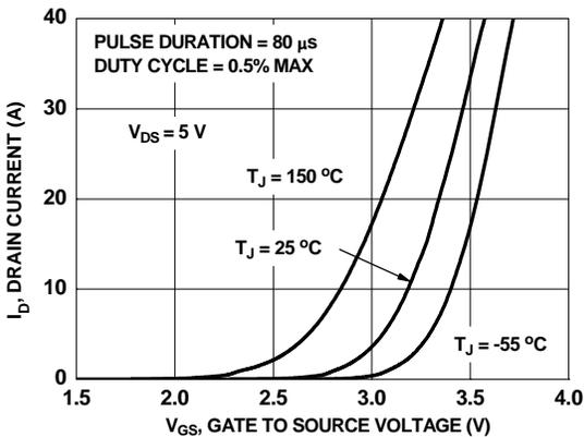
**Figure 5. Transfer Characteristics**
