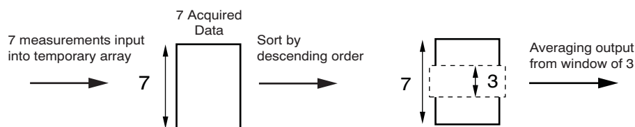
Figure 28. MAV Filter Operation (Patent Pending)
