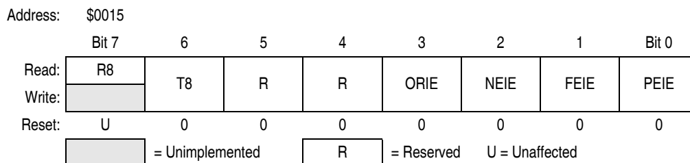
Figure 14-12. ESCI Control Register 3 (SCC3)
